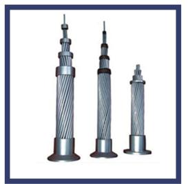
The mixed construction of ACSR makes it a very flexible medium from a design point of view. By varying the relative proportions of aluminium and steel the ideal conductor for any particular application can be produced. Generally, ACSR consists of a galvanized steel core of 1 wire, 7 wires or 19 wires surrounded by concentric layers of aluminium wire.
