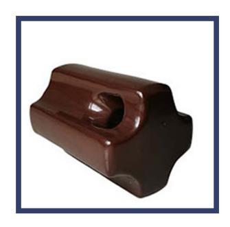
Normal system voltage: upto 11kV System highest voltage: upto 12.5kV 50 cycles dry flash over: upto 30kV 50 cycles wet flash over: upto 18kV Leakage distance: upto 80mm Tensile strength: upto 90kN
