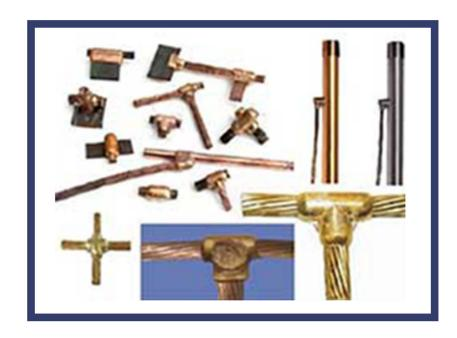
Exothermic welding is simple, cost efficient, self contained process of forming high quality connections. This process requires no external power or heat source making it completely portable. It uses high temperature reaction of powdered copper oxide and aluminium, within a mould, to form permanent connections.
